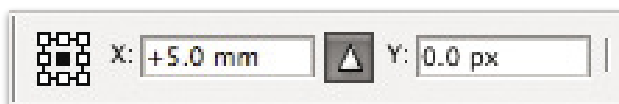
▲ The Free Transform command in Photoshop enables us to specify the movement of a layer or selection in any unit. Clicking on the triangle icon sets values relative to the object rather than to the canvas.
