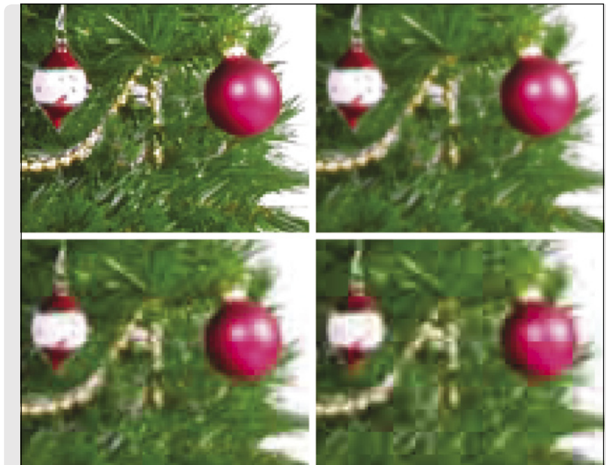
▲ Our original image (top left), greatly magnified, shows a lot of detail on this Christmas tree. Even at a high-quality Jpeg setting (top right), some fine detail is clearly lost in the leaves and ornaments. At a low setting (bottom left), we can start to see the 8 x 8 pixel blocks the Jpeg algorithm uses for compressing the image. At the lowest quality (bottom right) these blocks overpower the image.
